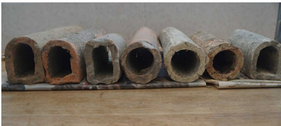
Figure1. A selection of field drains from an excavation at Lamp Hill, Wimpole (Photograph courtesy of Mike Coles).
