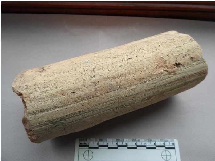
Figure 4. Section of ceramic drain pipe with extrusion lines visible (Authors photograph).
